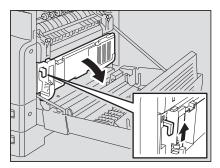
Remove the transfer charger cleaner from the front pocket of the transfer unit.
